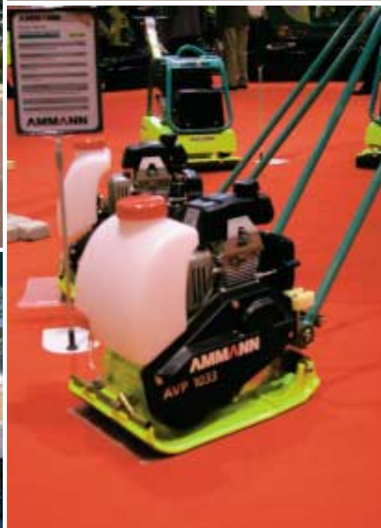
7. Amman asfalt handcompactor 1
